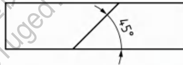
Figure 3 — Recommended method for joining the ends of the abrasive paper strip
