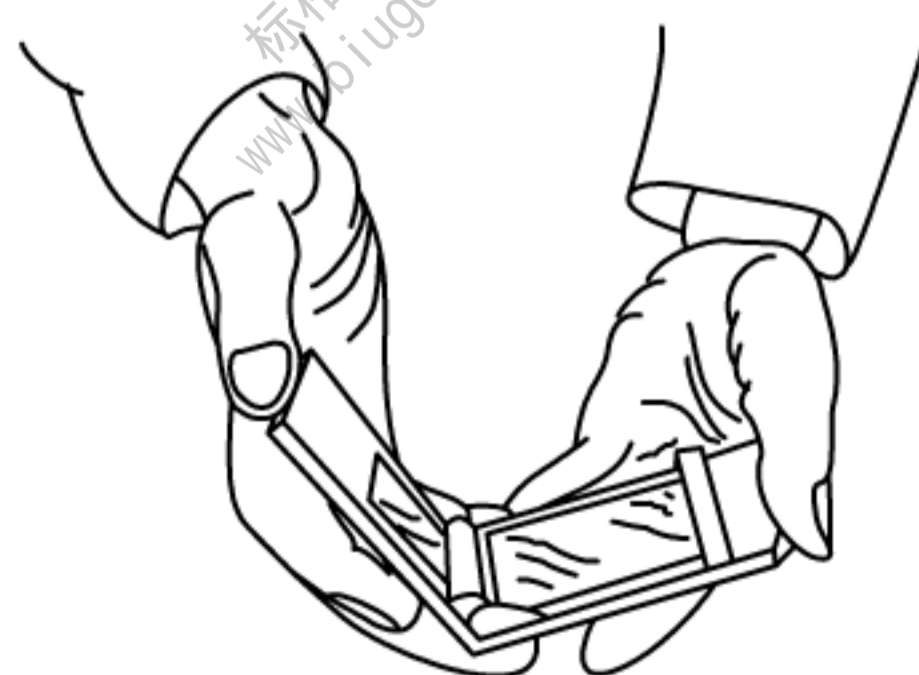
Figure 2 — Type 1 bend test apparatus in use
